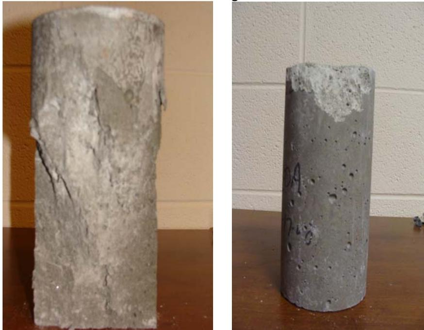
Photo for Sample No. 5B after Compressive Strength Test, Civil Eng. Lab, NCSU.
