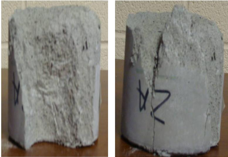
Photo for Sample No. 8AA after Compressive Strength Test, Civil Eng. Lab, NCSU.
