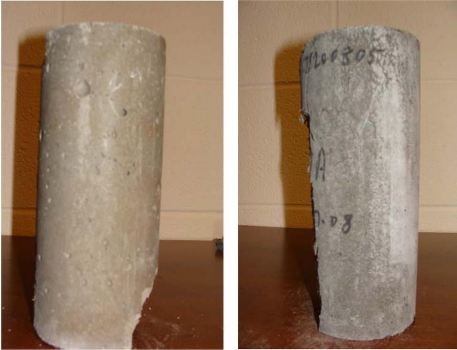
Photo for Sample No. 15A after Compressive Stress Test, Civil Eng. Lab, NCSU
