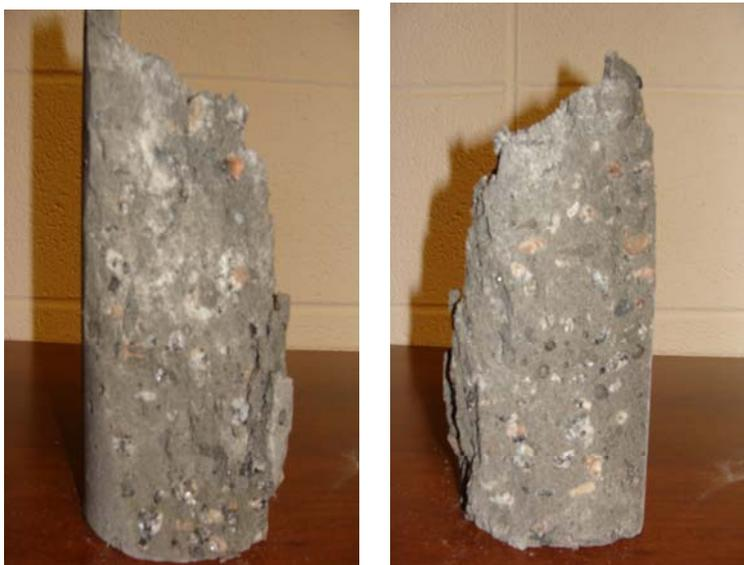
Photo for Sample No. 10A after Compressive Stress Test, Civil Eng. Lab, NCSU.
